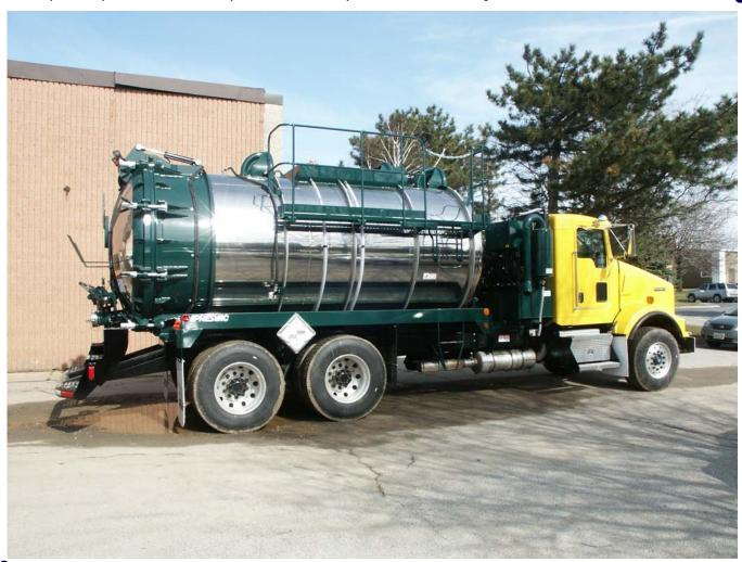
The Presvac Liquid Vac Dump is a versatile vacuum truck. It can be configured to suit a broad range of applications: collection and transport of hazardous and non-hazardous liquids, slurries and sludges, septic system cleaning, line jetting, material transfer, etc. The full opening door and large tipping angle make tank clean out an ease.
