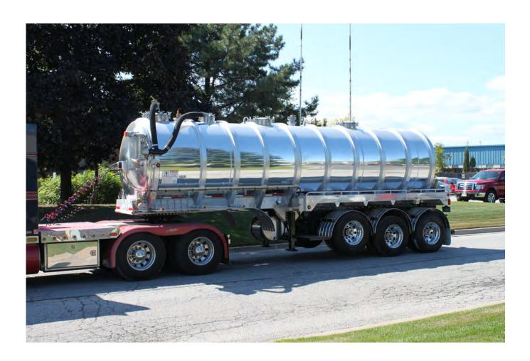
Presvac Aluminum Tank Trailers are designed strong. Extremely light weight vacuum loading / pressure off-loading on highway trailer. Multi-Compartment, numerous vacuum and water pump options provide unlimited versatility.
