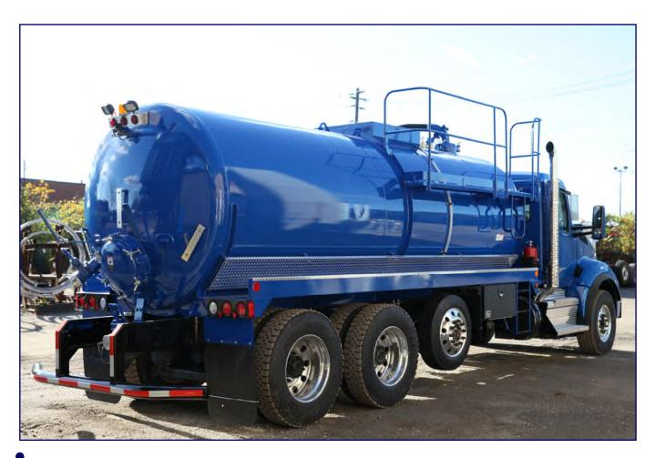
The Presvac Liquid Vac is a versatile vacuum truck. It can be configured to suit a broad range of applications: septic system cleaning, line jetting, collection and transport of hazardous and non-hazardous liquids, material transfer, etc.
