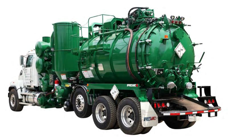
The Presvac Powervac is the ultimate PD Blower Wet / Dry Vacuum Loader. Operate as an air mover for dry applications or use full vacuum and extreme recovery rates for the toughest liquid, sludge and slurry jobs. The material knock out features in the Powervac debris tank minimize carry over. Heavy duty modular filtration configured to blower size and application provides superior blower protection and minimal maintenance.
