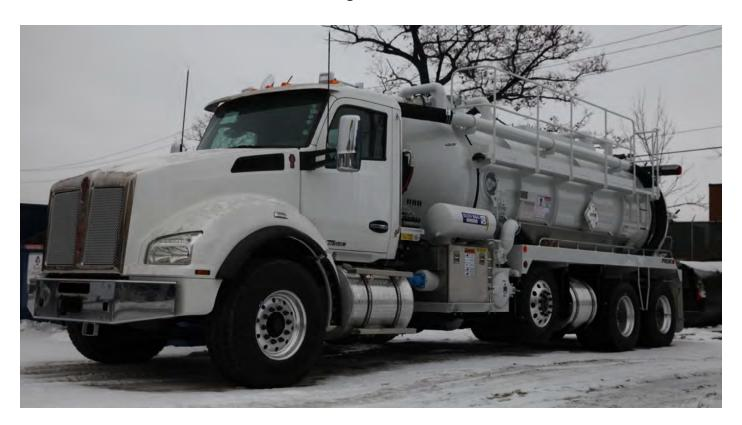
Designed for liquid, sludge and slurry applications with the added advantage of a PD Blower:
