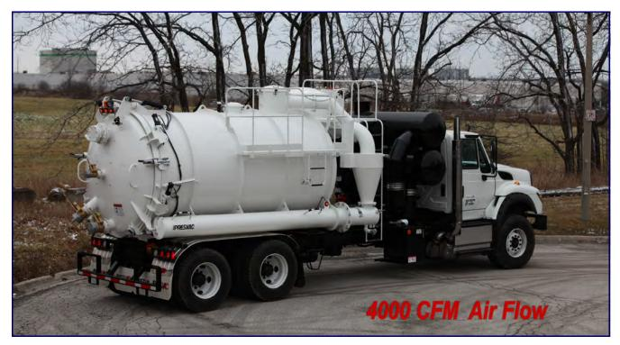
PD Blower: Hibon VTB840XL, Max. Vacuum: 28" HG, Free Air: 4000 CFM, 15"HG: 3400 CFM, 27" HG: 1600 CFM. Single Baghouse With 29 Bags, Single Cyclone, 12" Dump Chutes SS 304, Heavy Duty Spring Tensioned Bolts Allow For Adjustment To Maintain Leak Proof Sealing. Dump Chute Doors Open With Debris Tank Door.
