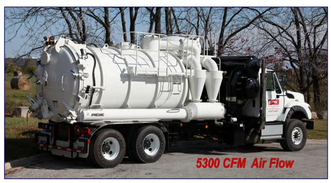
PD Blower: Hibon SIAV8702, Max. Vacuum: 28" HG, Free Air: 5300 CFM, 15"HG: 4700 CFM, 27" HG: 3000 CFM. Single Baghouse With 53 Bags, Two Cyclones, 12" Dump Chutes SS 304, Heavy Duty Spring Tensioned Bolts Allow For Adjustment To Maintain Leak Proof Sealing. Dump Chute Doors Open With Debris Tank Door.
